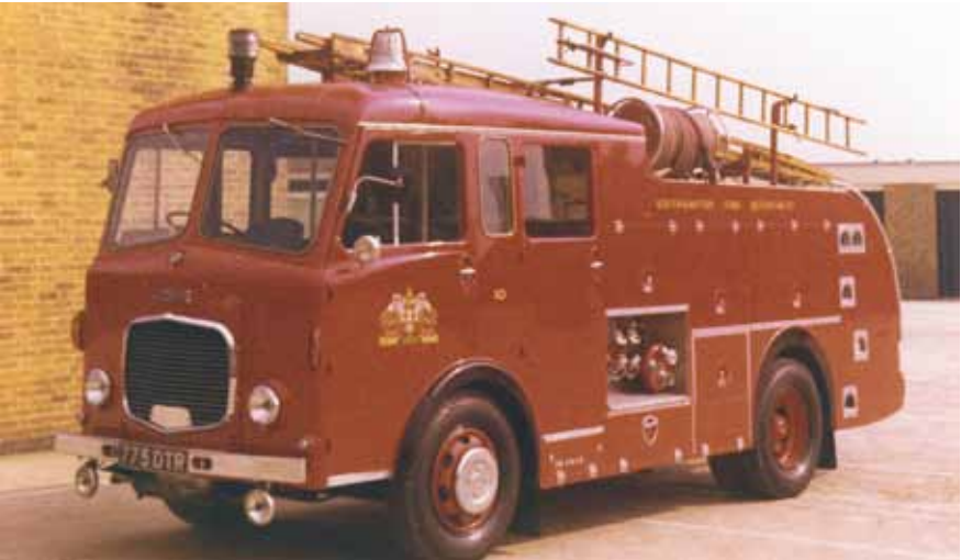
Dennis F24, 775 DTR, 'Number 10'. Purchased new by the Southampton Fire Brigade to serve as a spare Major Pump or Pump Escape. When used as a PE, the water in the tank was reduced from 300 gallons to 200 gallons.
