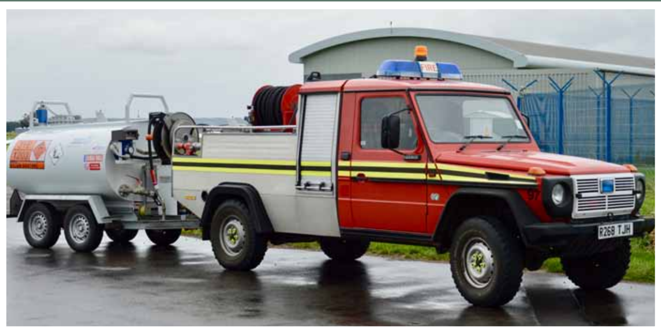
The former HMS Daedalus site, which had its own military fire service until it closed, now has this former Hampshire FRS (Lyndhurst and Brockenhurst) Steyr Puch Super G 'H4T' on the run as an RIV. The appliance was sold direct to the airport and HFRS Fleet Maintenance Centre completed foam installation and conversion from H4T to RIV.
