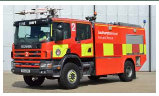
Southampton International Airport. Scania Rapid Intervention Vehicle. Built on a standard 4x4 truck chassis with bodywork completed by Carmichael, a name long associated with the fire service that is no longer in business.
