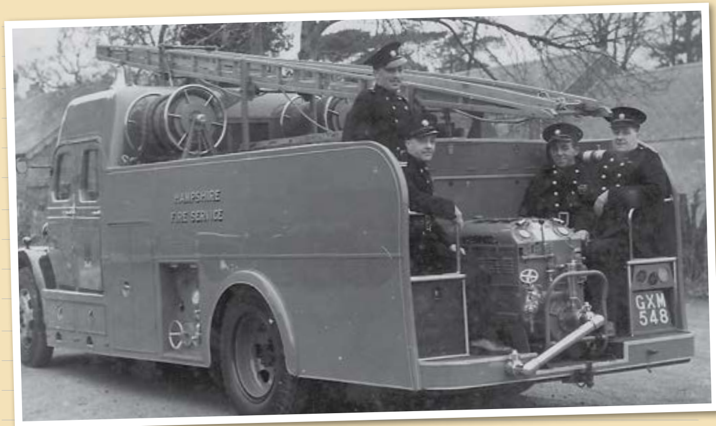
Sub O Fred Elliott and crew sat on newly converted Dodge Watertender, (Workshops conversion from a WW2 era 'Mobile Dam Unit'). On the side is a gear-driven hose-reel only pump, with the main pump at the back being a WW2 era Coventry Climax pump, which was originally designed to be slid from a trailer and wheeled wheelbarrow style. It this conversion, it could in fact be disconnected from the tank supply and taken to a water source. Two main jst achievable via a dividing breeching. And yes, crew members really did ride here if necessary – the days of riding 7. Photo probably 1950. Station may be Alresford??
